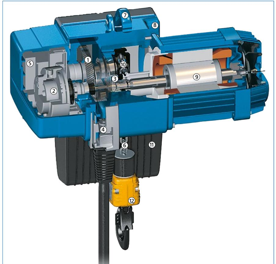
① **Gearbox** – maintenance-free for up to 10 years. With classification in FEM Group of Mechanisms Demag 2m+, the DC-Pro sets a new standard with a rated service life of 1900 hours at full load. In practical terms, this means the service life is extended by approx. 20 %. The helical gearing of all gearbox stages also reduces operating noise and provides for smooth operation.
